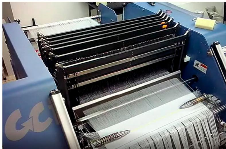
**Figure 4.** The laboratory harness loom during manufacturing of MLW.
