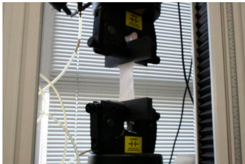
**Figure 5.** MLW sample during tensile test.
