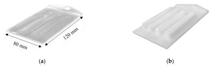
Figure 1. (a) Initial part thickness of 3 mm; (b) the extended ribs height 8.5 mm after cavity expansion.
