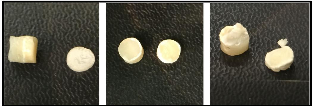
**Figure 6.** The failure modes after testing: adhesive failure (**left**), cohesive failure (**middle**), and mixed failure (**right**).
