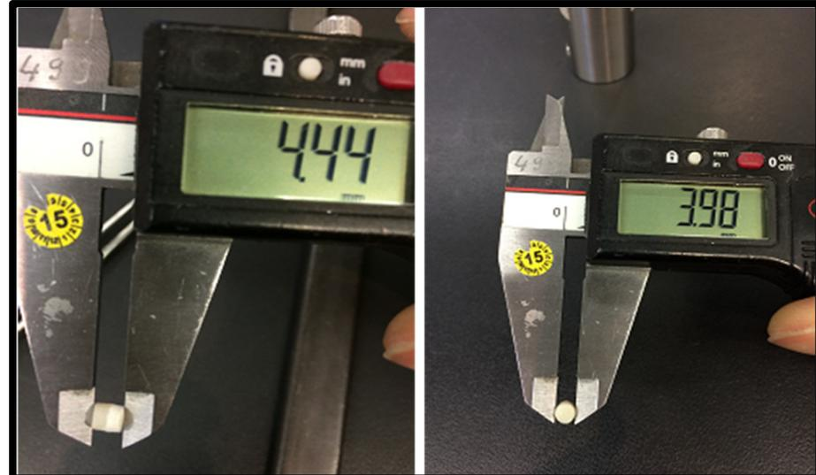
**Figure 2.** Calibration of the prepared restorative material samples.
