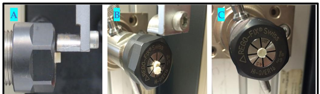
**Figure 5.** (A) Intact sample, (B) sample after force was applied, (C) junction of one restorative after testing.
