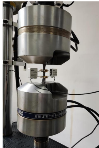
Figure 2. Clamping display of the specimen.
