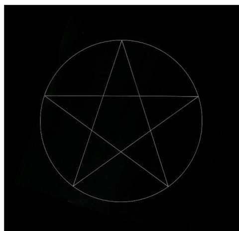
**Figure 7.** Result of laser scanning machining for large-area and consecutive pattern.
