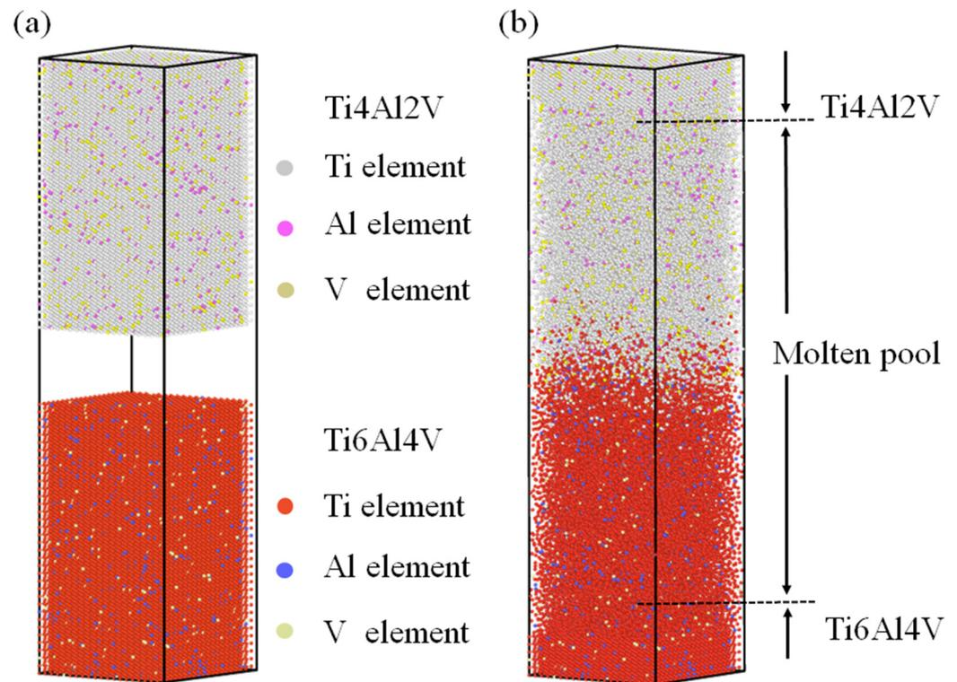
**Figure 1.** Welding model of TC4-TA17 dissimilar titanium alloy: (a) molecular dynamics calculation model before welding, in which the upper part is TC4 titanium alloy and the lower part is TA17 alloy; (b) molecular dynamics structure after welding, in which the middle is the molten pool area. The alloys form an obvious metallurgical bond.
