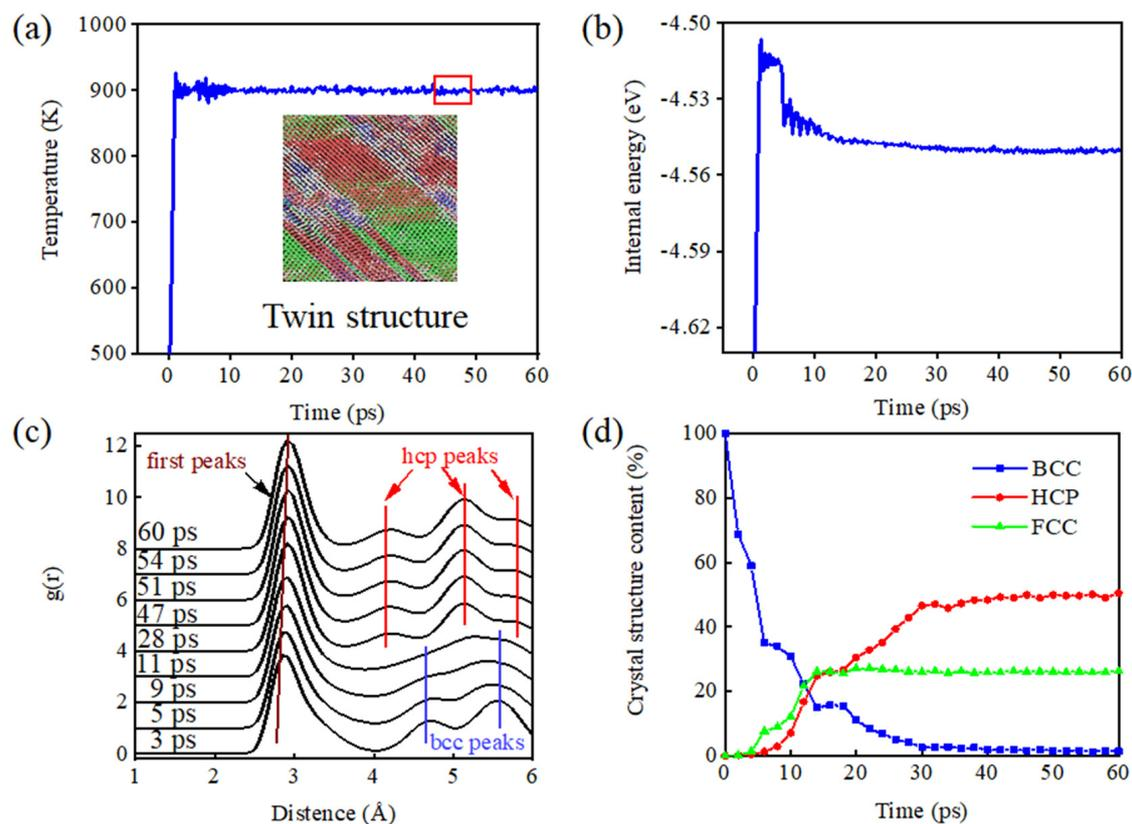
**Figure 2.** Microstructure of TC4 alloy after heat treatment and return to room temperature: (a) the relaxation process of the transformation from high-temperature face-centered cubic phase to low-temperature close-packed hexagonal phase finally forms a partial twin structure; (b) the change in binding energy during phase transformation; (c) the radial distribution function during phase transformation; and (d) analysis of the relative contents of each phase.
