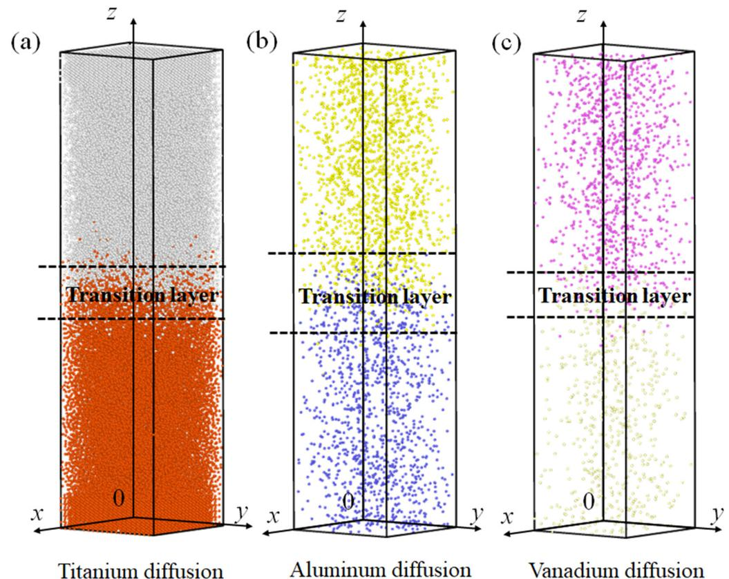
**Figure 5.** Analysis of the TC4-TA17 dissimilar titanium alloy welding diffusion layer: (a–c) diffusion layer structures of Al, Ti, and V atoms, respectively.
