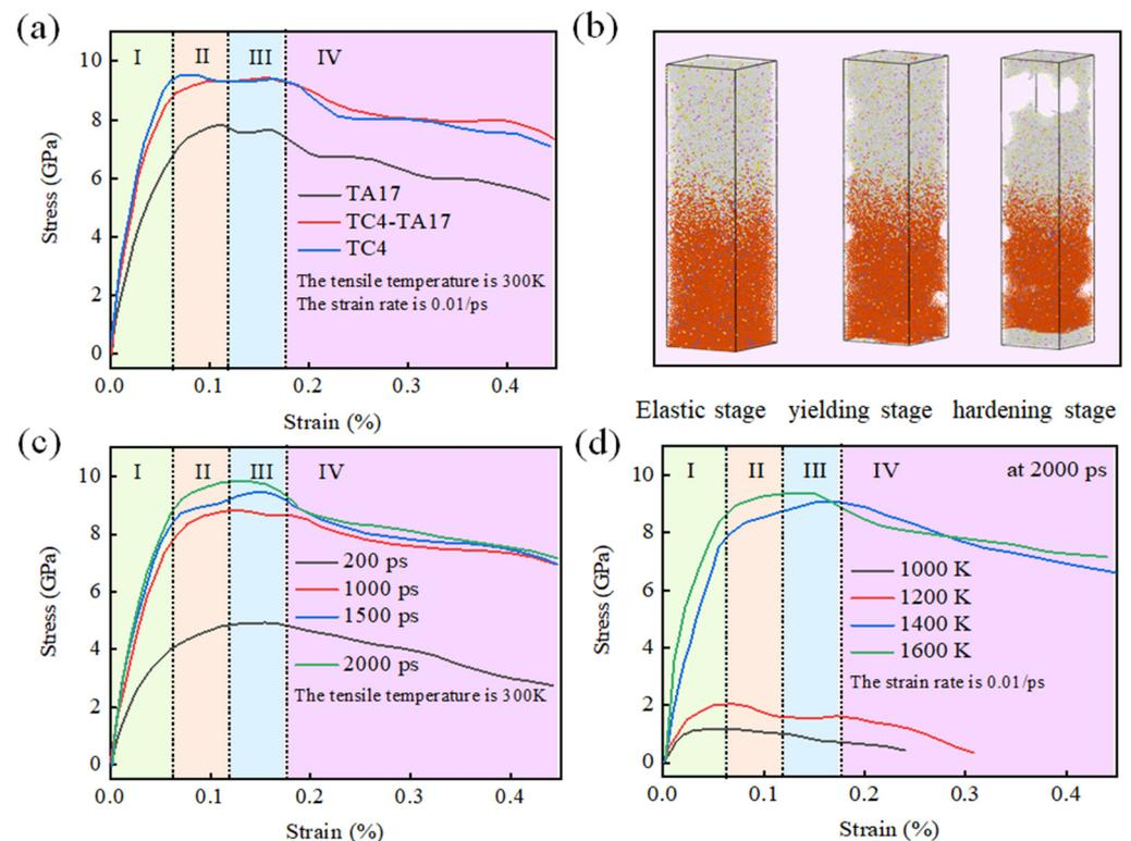
**Figure 7.** Fracture characteristics and fracture mechanism analysis of TC4-TA17 dissimilar titanium alloy after welding: (a) fracture characteristics of TC4-TA17 dissimilar titanium alloy at the tensile temperature is 300 K and the strain rate is 0.01/ps; and (b) fracture mechanism; (c) strain rate (the tensile temperature of 300 K); and (d) effect of holding temperature on tensile properties (the strain rate is 0.01/ps).
