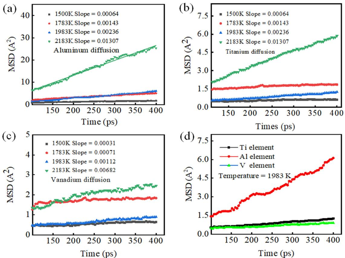
**Figure 4.** Diffusion mechanism of Al, Ti, and V atoms during welding: (a–c) root-mean-square displacements of Al, Ti, and V atoms at different temperatures; (d) root-mean-square displacements of Al, Ti, and V atoms at 1983 K.
