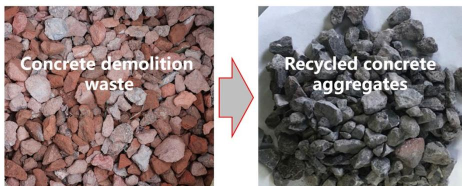
**Figure 1.** The recycled concrete aggregates were selected from the concrete demolition waste.
