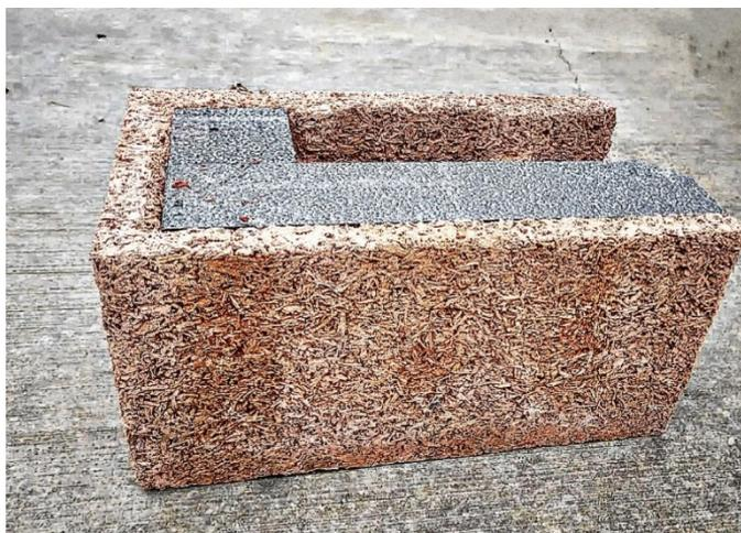
**Figure 1.** Concrete block with wood chips.
