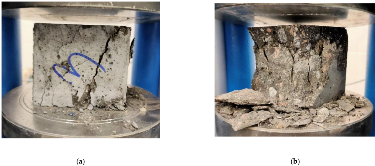
Figure 13. Compression Strength Failure Shapes: (a) Basalt Fiber reinforced High-Performance Concrete PC; (b) High-Performance Concrete.
