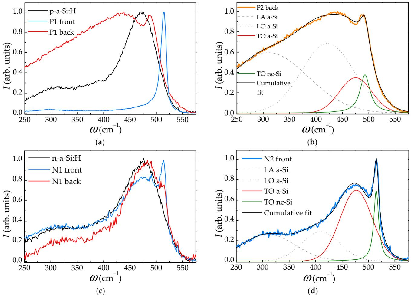
**Figure 6.** (a) Typical Raman spectra for the initial p-a-Si film and irradiated region P1. (b) Decomposition of the Raman spectrum obtained from the back of the sample P2. (c) Typical Raman spectra for the initial n-a-Si film and irradiated region N1. (d) Decomposition of the Raman spectrum for the front of the sample N2. All spectra are normalized by maximum intensity.
