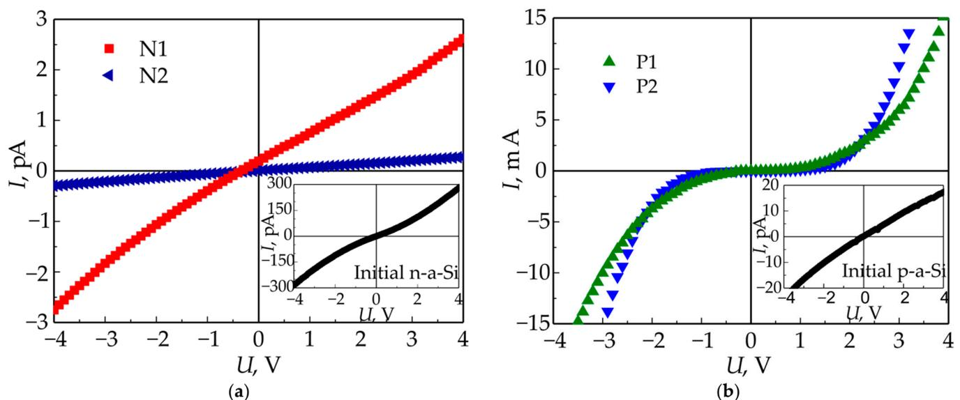
**Figure 7.** (a) CVC of irradiated p-a-Si films. (b) CVC of irradiated n-a-Si films. The insets show the CVC of the initial p-a-Si and n-a-Si films, respectively.
