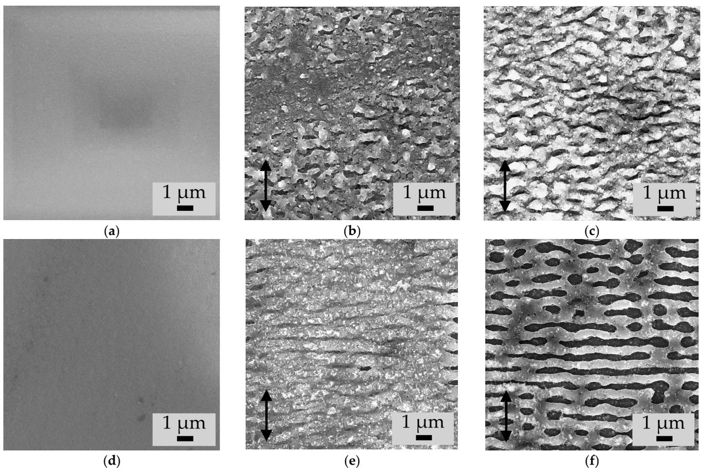
**Figure 4.** SEM images of the surfaces of (a) initial p-a-Si; femtosecond laser-irradiated samples (b) P1, (c) P2; (d) initial n-a-Si; femtosecond laser-irradiated samples (e) N1 and (f) N2. The direction of laser polarization is indicated by an arrow on the images.
