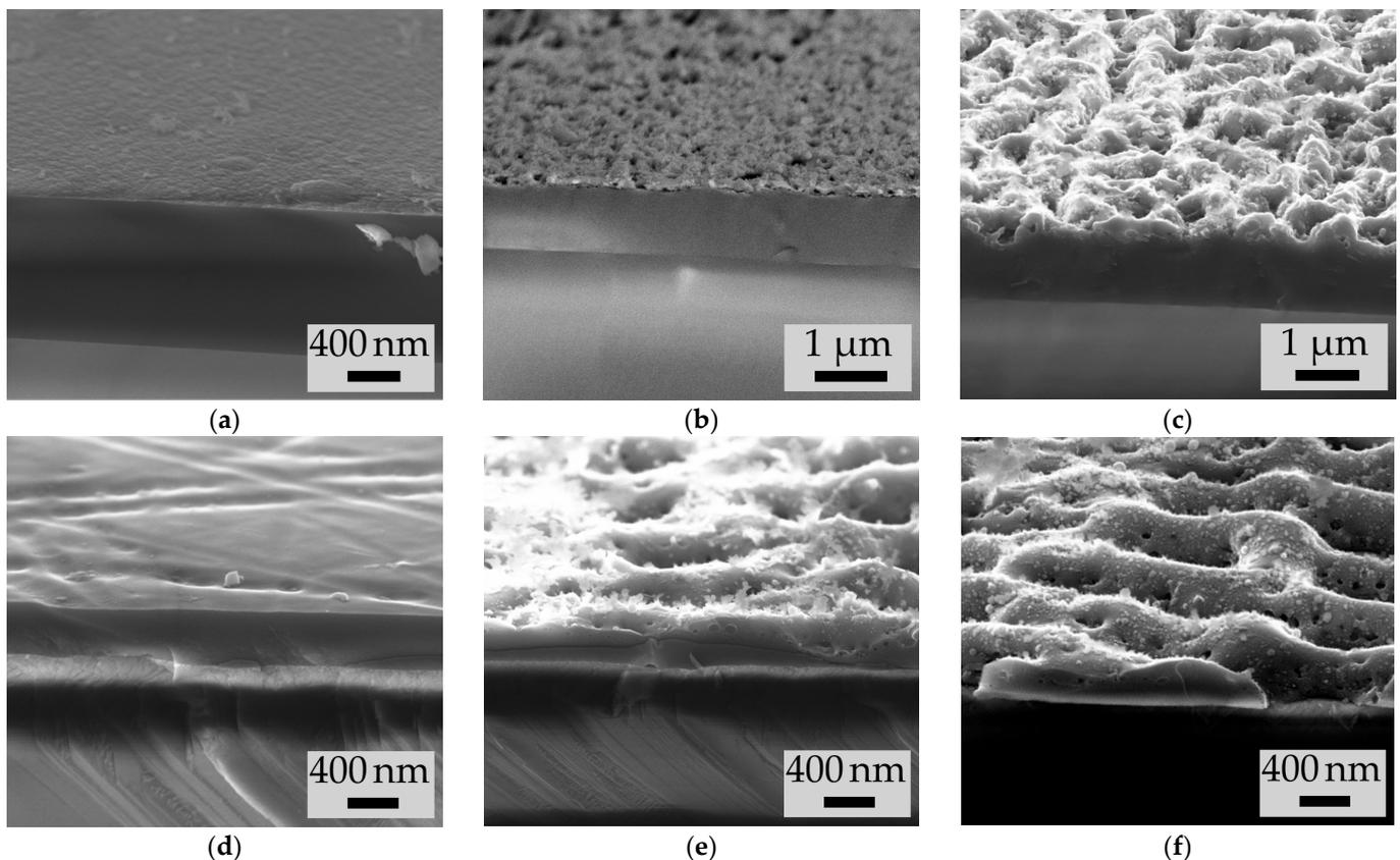
**Figure 5.** SEM images of the cross sections of the samples (a) unirradiated p-a-Si (b) P1, (c) P2, (d) unirradiated n-a-Si (e) N1 and (f) N2, obtained at a 10° angle to the cross section surface.
