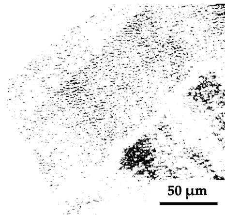
**Figure 3.** Image of the p-a-Si surface irradiated with  $N = 200$ , obtained by optical microscope in transmission mode. Dark sites are silicon isles surrounded by empty space, arisen because of complete film ablation.
