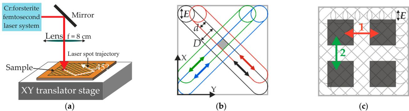
**Figure 2.** (a) Scheme of experimental setup used to process the a-Si films by femtosecond laser pulses. (b) Scanning mode template of femtosecond laser irradiation. Four different laser beam passes are indicated by black, red, green, and blue colors. The arrow  $E$  indicates laser polarization. (c) Scheme of the electrical contacts (gray squares) on the irradiated sample.
