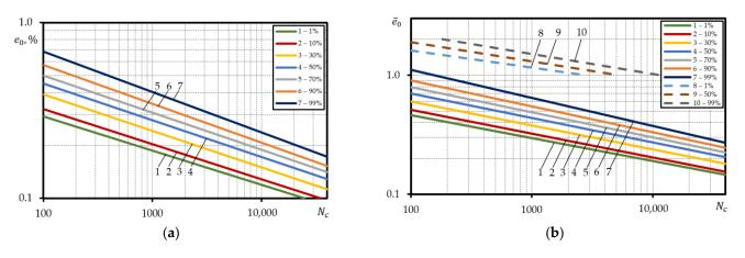
**Figure 10.** Probabilistic low-cycle fatigue curves under strain-controlled loading for aluminium alloy D16T1 built using: the absolute coordinates (**a**); the relative coordinates (**b**); straight lines—calculated, dashed lines—experiment.
