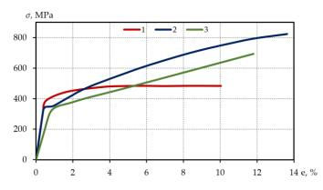
**Figure 1.** Single uniaxial tensile deformation curves: 1—aluminium alloy D16T, 2—structural steel C45, 3—alloyed steel 15Cr2MoVA.
