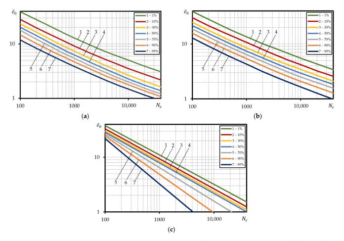
**Figure 7.** Calculated probabilistic low-cycle fatigue curves under strain-controlled loading for steel 15Cr2MoVA, built in the relative coordinates, according to: (a)—Equation (3), (b)—Equation (5), (c)—Equation (6).
