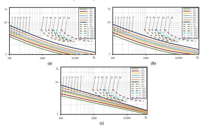
**Figure 9.** Comparison of the calculated probabilistic low-cycle fatigue curves under strain-controlled loading with the experimental ones for steel C45; straight lines—calculated, dashed lines—experiment; according to: (a)—Equation (3), (b)—Equation (5), (c)—Equation (6).
