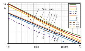
**Figure 11.** Comparison of the probabilistic low-cycle fatigue curves calculated under strain-controlled loading with the experimental ones for steel 15Cr2MoVA; straight lines—calculated, dashed lines–experiment; normalized characteristic according to: 1—Equation (3), 2—Equation (5), 3—Equation (6); reference characteristics, according to: 1'—Equation (3), 2'—Equation (5), 3'—Equation (6); calculated, according to: 4—Equation (3)  $n_e = 2$ , 5—Equation (3)  $n_N = 10$ .
