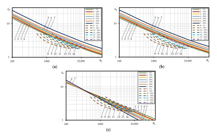
**Figure 8.** Comparison of the calculated probabilistic low-cycle fatigue curves under strain-controlled loading with the experimental ones for steel 115Cr2MoVA; straight lines—calculated, dashed lines—experiment; according to: (**a**)—Equation (3), (**b**)—Equation (5), (**c**)—Equation (6).
