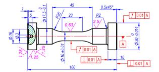
Figure 2. Specimens for low-cycle fatigue experiments (units in mm).
