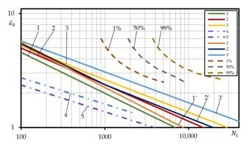
**Figure 12.** Comparison of the probabilistic low-cycle fatigue curves calculated under strain-controlled loading with the experimental ones for steel C45; straight lines—calculated, dashed lines– experiment; normalized characteristic according to: 1—Equation (3), 2—Equation (5), 3—Equation (6); reference characteristics, according to: 1′—Equation (3), 2′—Equation (5), 3′—Equation (6); calculated, according to: 4—Equation (3) if  $n_e = 2$ , 5—Equation (3) if  $n_N = 10$ .
