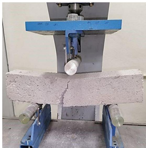
**Figure 6.** Apparatus for three-point bending test.
