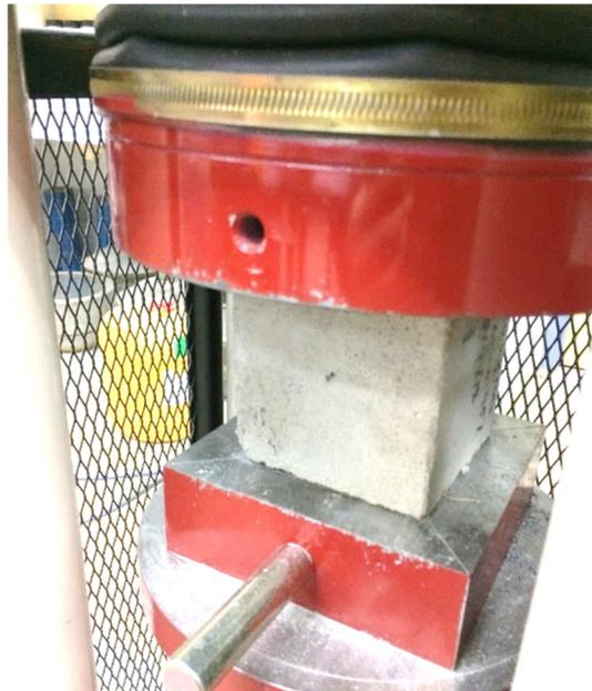
**Figure 5.** Setup for compression test.
