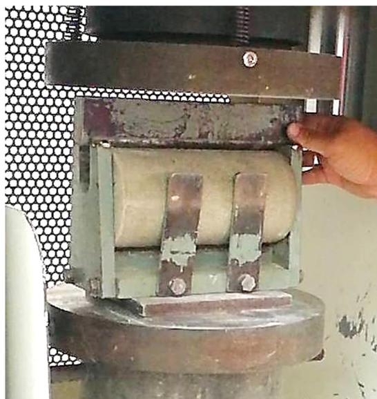
Figure 7. Splitting tensile test apparatus.
