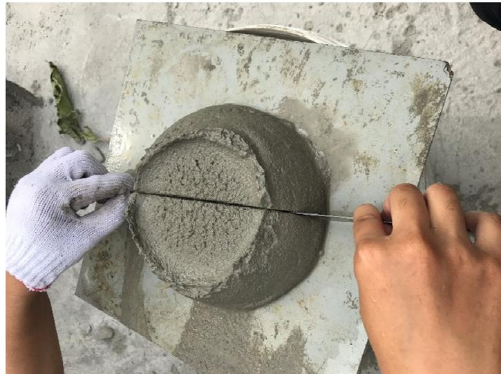
**Figure 3.** Measurement of the spreadability of foamed concrete.
