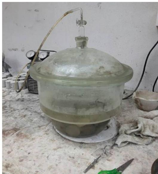
**Figure 4.** Vacuum saturation procedure.
