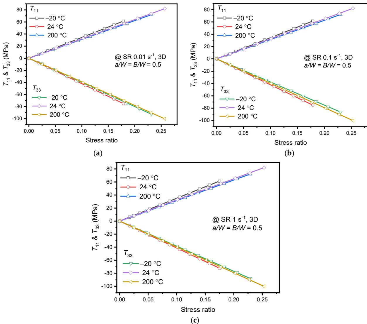
**Figure 10.**  $T_{11}$  and  $T_{33}$  at specimen thickness center obtained using FEA for different temperature vs. Stress ratio (a)  $0.01\text{ s}^{-1}$ ; (b)  $0.1\text{ s}^{-1}$ ; (c)  $1\text{ s}^{-1}$ .
