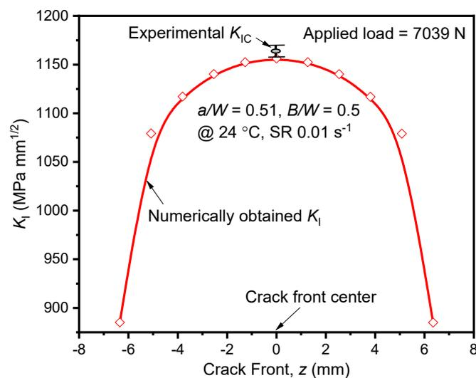
**Figure 6.** Stress intensity factor ( $K_I$ ) along the crack front at  $24 \text{ }^\circ\text{C}$ .
