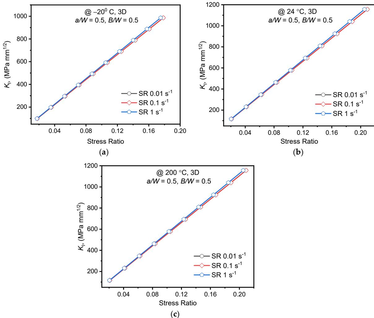
**Figure 7.**  $K_I$  at specimen thickness center obtained using FEA for different strain rates vs. Stress ratio (a) @ -20 °C; (b) 24 °C; (c) 200 °C.
