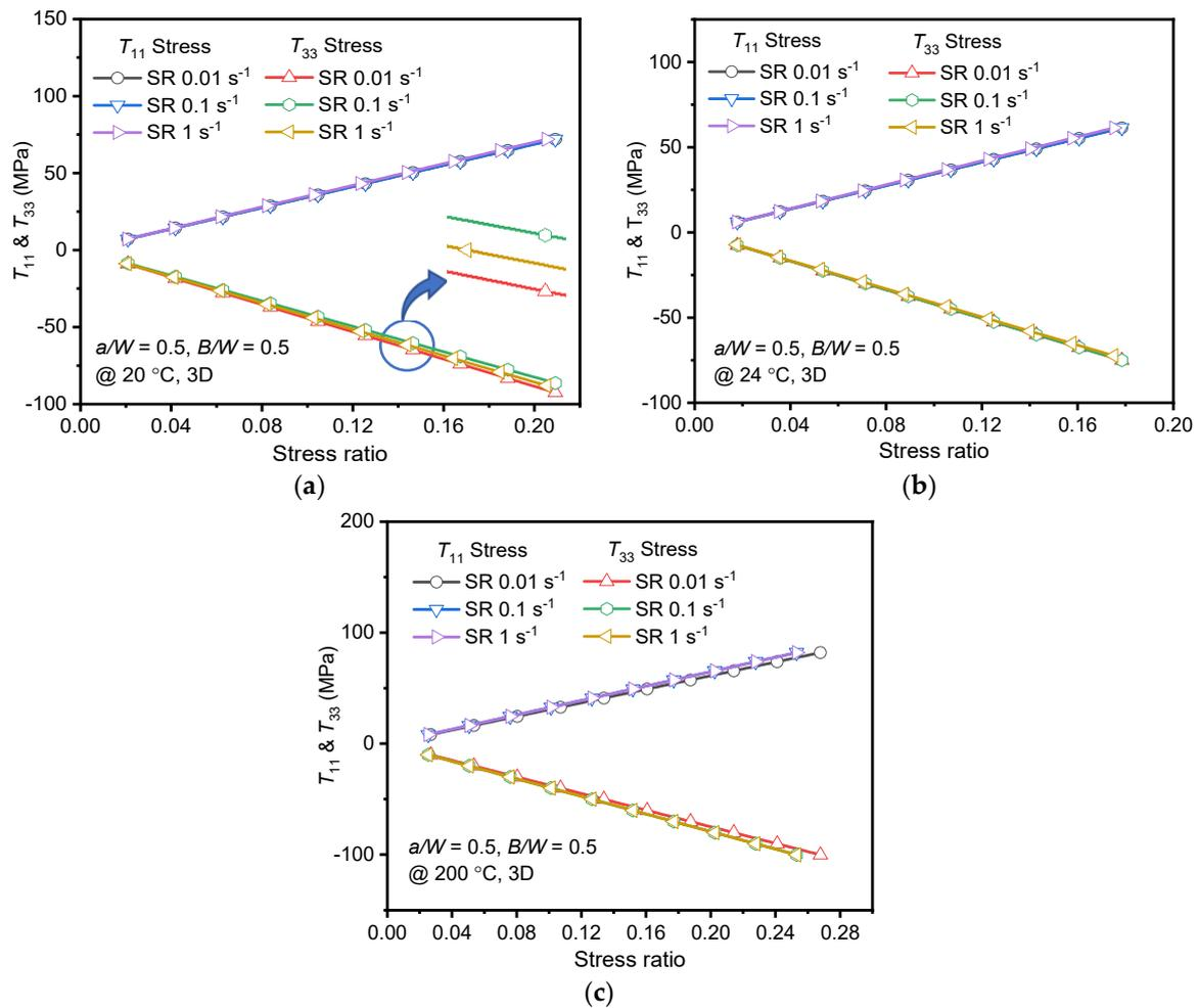
**Figure 8.**  $T_{11}$  and  $T_{33}$  at specimen thickness center obtained using FEA for different strain rates vs. Stress ratio (a) @  $-20\text{ }^{\circ}\text{C}$ ; (b)  $24\text{ }^{\circ}\text{C}$ ; (c)  $200\text{ }^{\circ}\text{C}$ .
