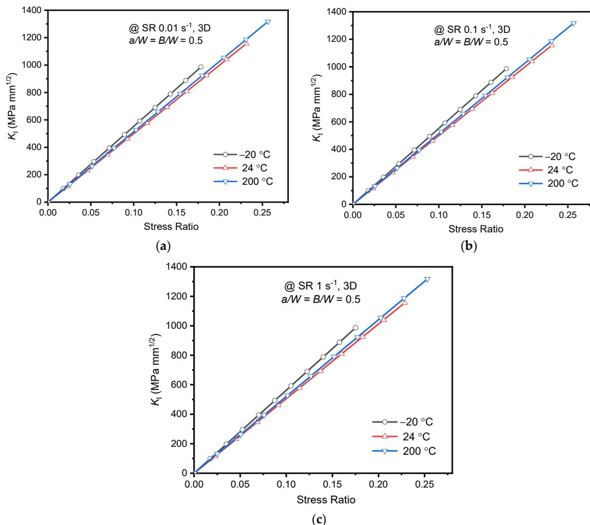
**Figure 9.**  $K_I$  at specimen thickness center obtained using FEA for different temperature vs. Stress ratio (a) SR 0.01 s<sup>−1</sup>; (b) SR 0.1 s<sup>−1</sup>; (c) SR 1 s<sup>−1</sup>.
