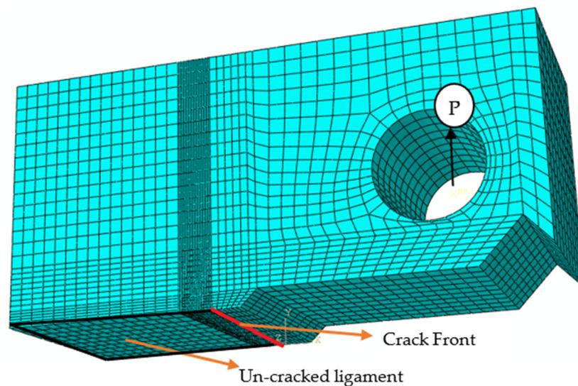
**Figure 3.** C(T) Meshed Model with Boundary conditions.
