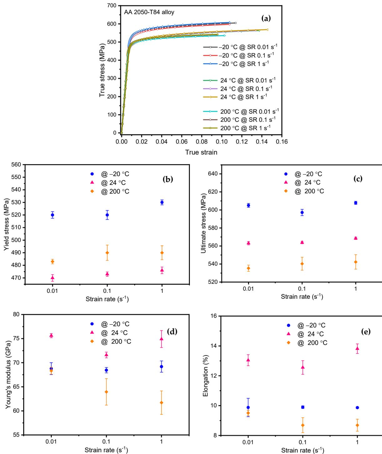
**Figure 4.** Strain rate and Temperature effect on: (a) True stress-strain curves (b) Yield stress; (c) Ultimate stress; (d) Young's modulus; (e) elongation.
