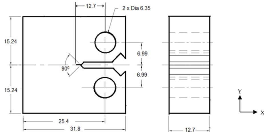
**Figure 2.** Compact Tension (C(T)) Specimen. All dimensions are in mm.
