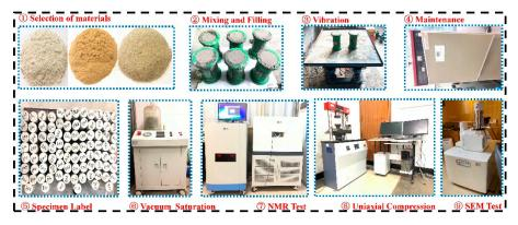
Figure 1. Specimen making and testing.
