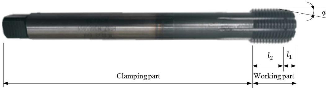
Figure 2. Structure of extrusion tap.
