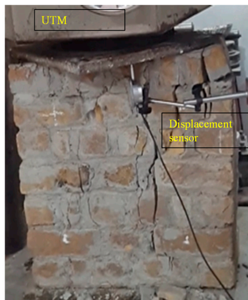
Figure 4. Experimental setup for the compressive strength of prism.
