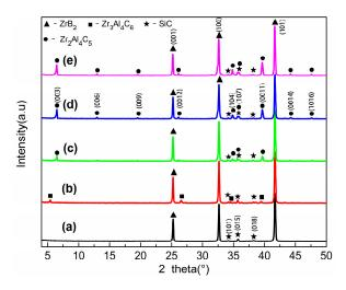
**Figure 2.** XRD patterns of composite ceramics at different Zr<sub>2</sub>Al<sub>4</sub>C<sub>5</sub> contents: (**a**) ZAC0, (**b**) ZAC10, (**c**) ZAC20, (**d**) ZAC30, (**e**) ZAC40.
