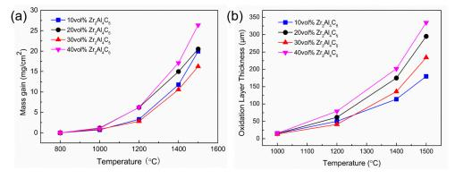
**Figure 6.** (a) Changes of oxidative weight gain and (b) oxidation layer thickness of samples at different contents of  $Zr_2Al_4C_5$ .
