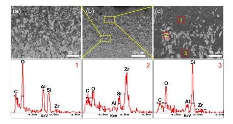
**Figure 12.** BESEM and EDS micrographs of the oxide layer section of the ZAC30 specimen after oxidation at 1500 °C for 30 min (**a**–**c**). (**a**,**c**) magnified SEM images of the areas enclosed in yellow dotted rectangles in (**b**).
