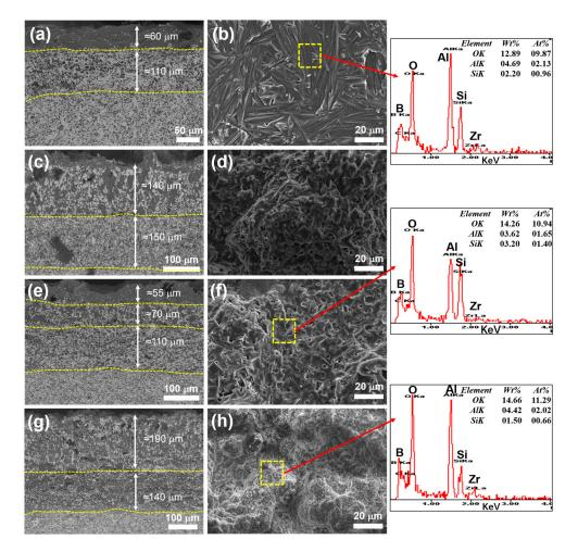
**Figure 10.** SEM and EDS pictures of the cross section and surface of the samples after oxidation at 1200 °C for 30 min: (**a**,**b**) ZAC10, (**c**,**d**) ZAC20, (**e**,**f**) ZAC30, (**g**,**h**) ZAC40.
