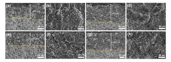
**Figure 9.** SEM pictures of the cross section and surface of the samples after oxidation at 1200 °C for 30 min: (**a**,**b**) ZAC10, (**c**,**d**) ZAC20, (**e**,**f**) ZAC30, (**g**,**h**) ZAC40.
