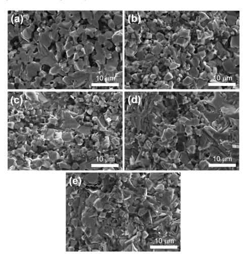
fractures. With the increase of  $Zr_2Al_4C_5$  content, the roughness degree increased and the grain size of  $ZrB_2$  gradually decreased, as shown in Table 1.
