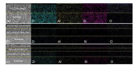
**Figure 11.** EDS pattern of the ZAC30 sample at different oxidation temperatures: (**a**) 1200 °C, (**b**) 1400 °C, (**c**) 1500 °C.
