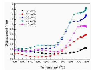
Figure 1. Displacement curve of pressure punch at different temperatures.
