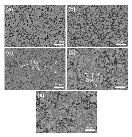
**Figure 3.** Backscattered electron phase pictures of polished surfaces of multi-phase ceramics at different  $Zr_2Al_4C_5$  contents: (a) ZAC0, (b) ZAC10, (c) ZAC20, (d) ZAC30, (e) ZAC40.
