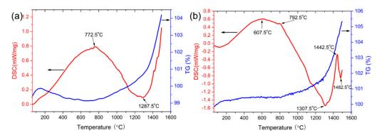
**Figure 7.** TG–DSC curve of multi-phase ceramics: (**a**) ZAC30, (**b**) ZAC40. Red line is differential scanning calorimetry, blue line is thermogravimetry.
