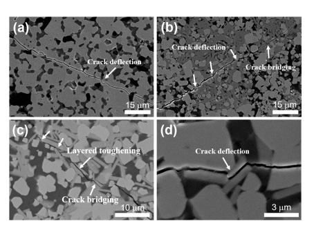
**Figure 5.** Expansion path diagram of the crack tip of multi-phase ceramics: (**a**) ZAC0, (**b**) ZAC20, (**c**) ZAC30, (**d**) ZAC30.
