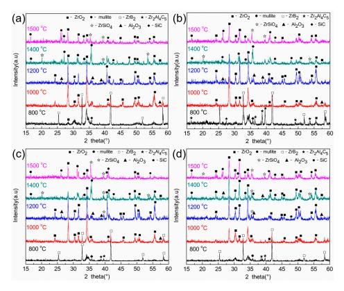
**Figure 8.** XRD patterns of composite ceramics oxidized for 30min at different oxidation temperatures: (a) ZAC10, (b) ZAC20, (c) ZAC30, (d) ZAC40.
