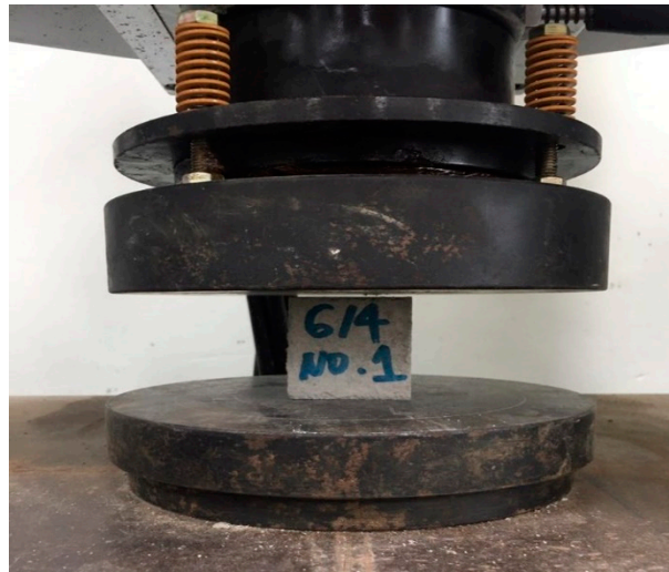
Figure 4. The compressive strength test setup.
