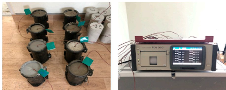
Figure 3. The heat of hydration measurement.
