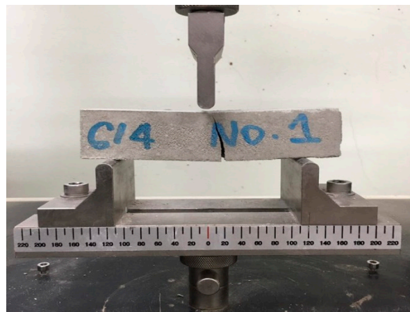
Figure 5. The flexural strength test setup.
