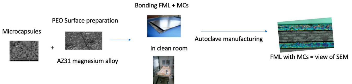
**Figure 2.** Scheme of FML manufacturing.
