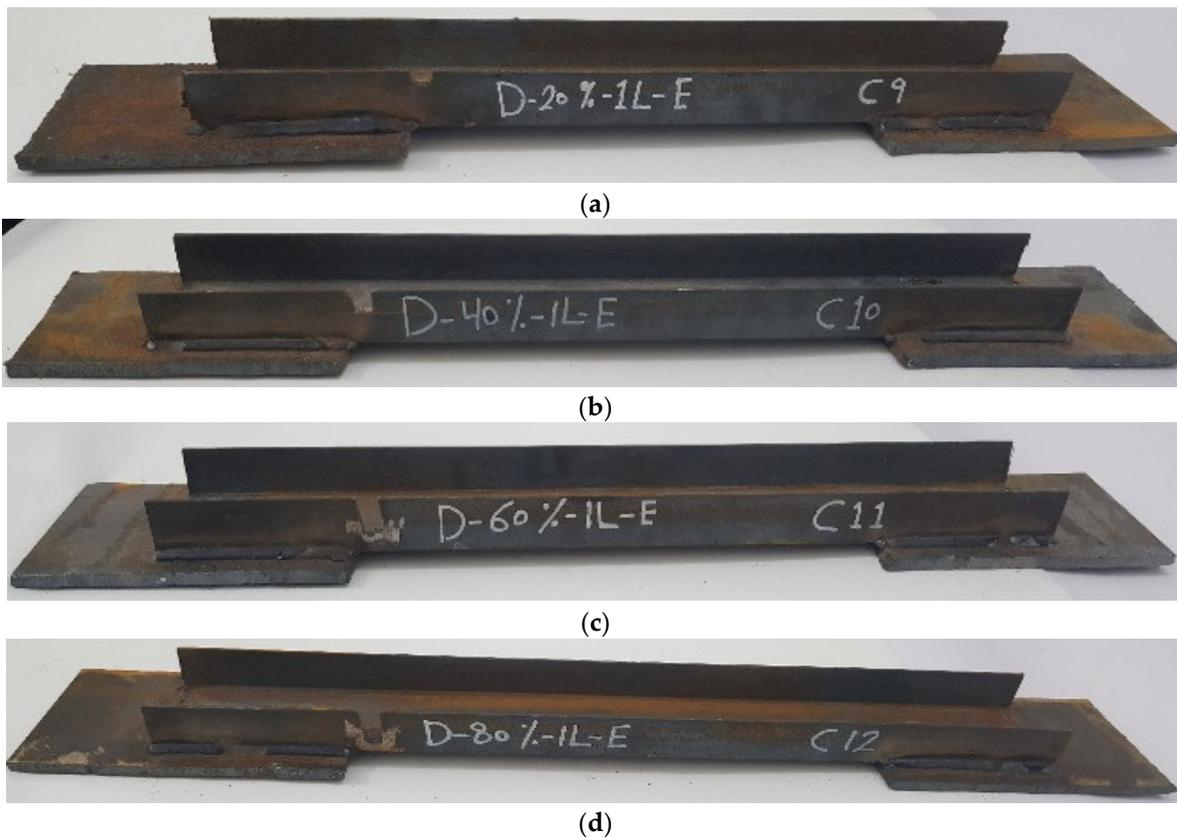
**Figure 5.** The shape of the third group with damage in one leg at the end of the element's length: (a) D-20%-1L-E; (b) D-40%-1L-E; (c) D-60%-1L-E; (d) D-80%-1L-E.
