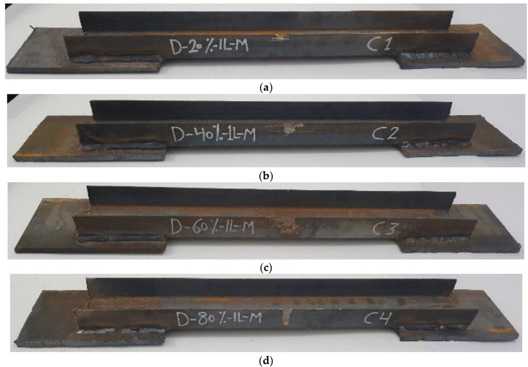
**Figure 3.** The shape of the first group with damage in one leg in the middle of the element's length: (a) D-20%-1L-M; (b) D-40%-1L-M; (c) D-60%-1L-M; (d) D-80%-1L-M.
