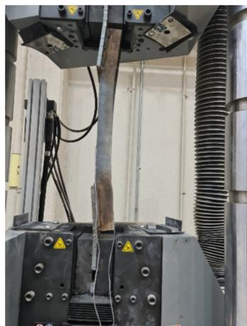
**Figure 7.** The method of attaching the sample to the tension machine employed in the tests.
