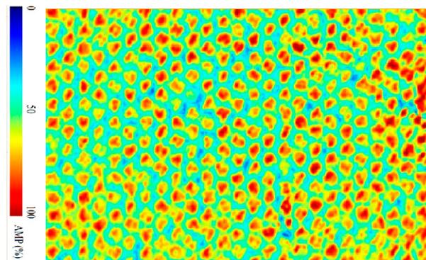
**Figure 3.** Ultrasonic scanning result of no initial damage in specimen.
