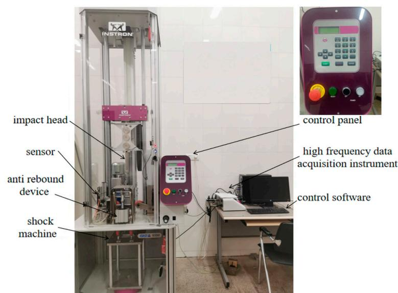
**Figure 2.** Impact test machine.
