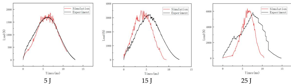
**Figure 8.** Load–time curves at different impact energies.
