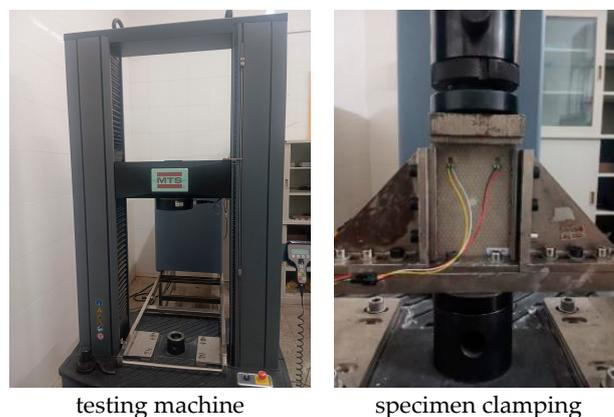
**Figure 13.** Compression test.
