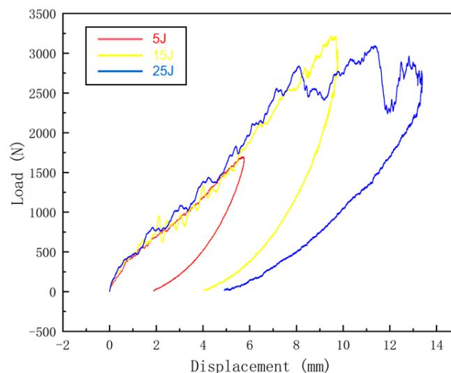
**Figure 4.** Load–displacement curves at different impact energies.
