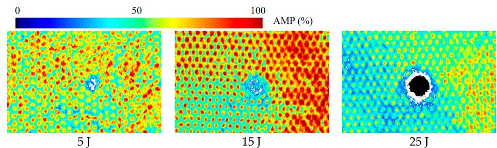
**Figure 5.** C-scan results of damaged specimens.
