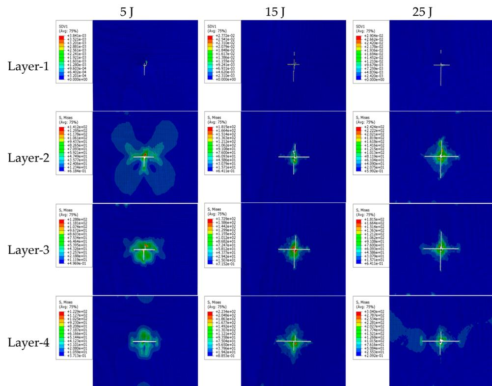
Figure 9. Damage nephogram at various impact energies.
