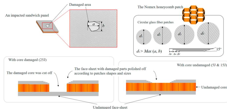
Figure 12. Repair schematic diagram.
