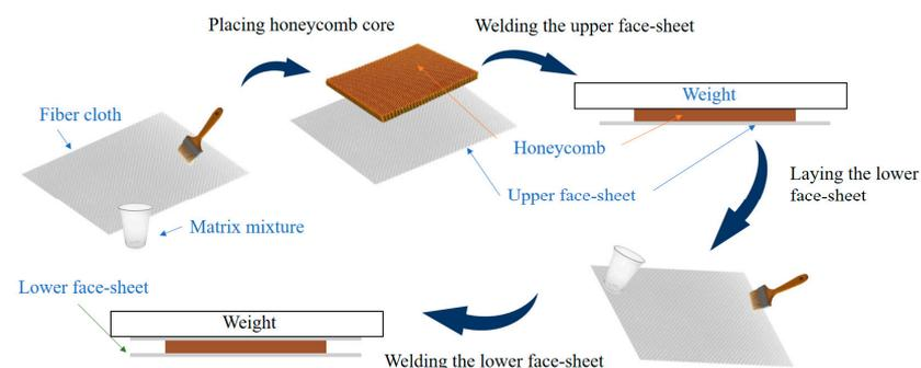
**Figure 1.** Manufacturing process.
