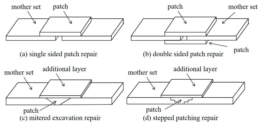
Figure 11. Typical adhesive repair types.
