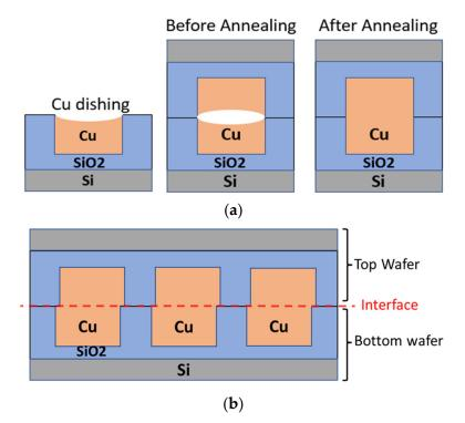
**Figure 1.** (a) Schematic drawing of hybrid bonding process flow. (b) Schematic drawing of misalignment at the bonding interface between the top wafer and bottom wafer.
