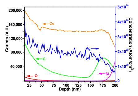
**Figure 4.** SIMS depth profile for a sample deposited with 4 DCs. The left axis shows the signal counts, whereas the right axis shows the Ag concentration determined using an implanted standard.
