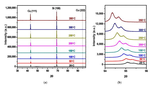
**Figure 10.** High-temperature XRD patterns of Cu(Ag) alloy films with 1.25% Ag obtained at different temperatures where: (**a**) the peak at 43.2° corresponds to Cu(111) and the one at 69.25° corresponds to Si(100) from the substrate; (**b**) zoomed-in view of the Cu (222) XRD peak at 95° showing a systematic shift in the Cu(222) peak towards lower angles with increasing temperature.
