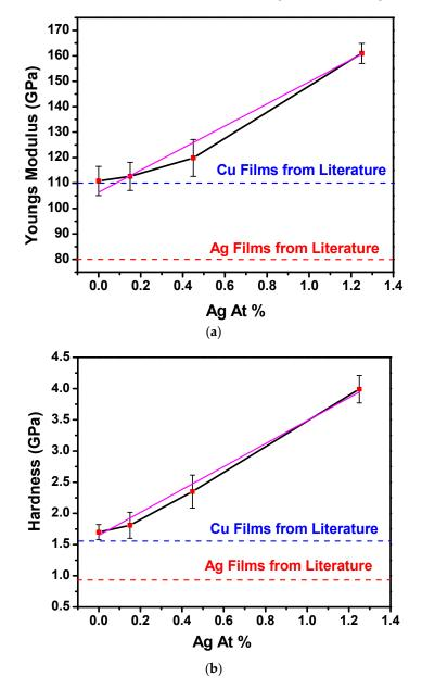
**Figure 9.** (a). Modulus vs. Ag content of the Cu(Ag) alloy films showing the modulus values linearly increasing with the increase in the Ag content of the films. (b). Hardness vs. Ag content of the Cu(Ag) alloy films showing the hardness values linearly increasing with the increase in the Ag content of the films. Black lines connect mean values, with linear fit plotted in purple.
