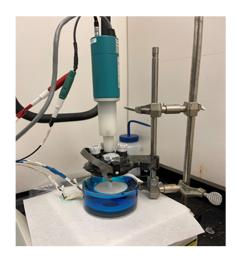
Figure 3. Reaction setup used for electrodeposition.
