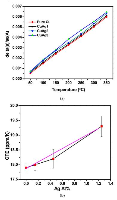
**Figure 11.** (a). Temperature dependence of the ratio of change in the lattice parameter compared to the original value. (b). The calculated CTE vs. Ag content depicts a linear dependence on composition. Black lines connect mean CTE values, with a linear fit plotted in purple.
