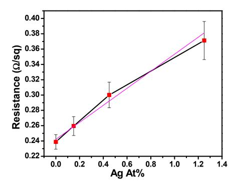
**Figure 12.** Sheet resistance vs. the Ag content of Cu(Ag) films showing that with an increase in the Ag content of the Cu(Ag) films, the sheet resistance also increases linearly. Black line connects means of data, with linear fit plotted in purple.
