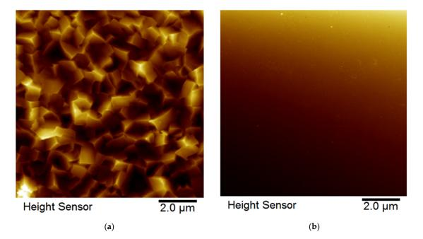
**Figure 8.** Surface roughness measured by AFM: (**a**) for an as-deposited sample using 4 DCs showing a significantly rough surface and (**b**) smooth surface obtained after CMP polishing.
