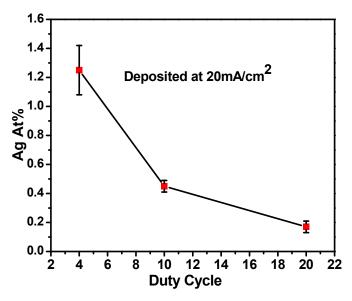
**Figure 5.** Ag content vs. duty cycle for films deposited with a current density of 20 mA/cm<sup>2</sup>. As anticipated, a lower duty cycle allows for a longer window for the displacement reaction, resulting in higher Ag incorporation.
