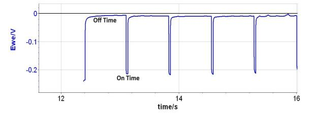
Figure 2. Example of the pulse plating profile used for the deposition of Cu(Ag) alloys.
