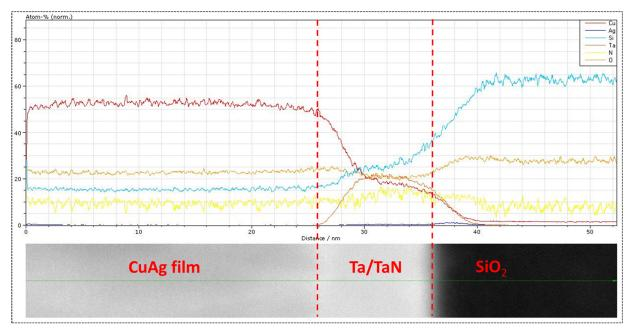
**Figure 7.** EDS line scan for Cu(Ag) alloy film deposited at 4 DCs showing a uniform concentration of Cu and Ag with no periodic banding or peaks.
