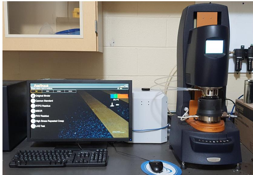
**Figure 6.** The dynamic shear rheometer.
