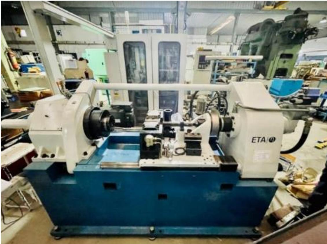
**Figure 1.** Rotary friction welding setup.
