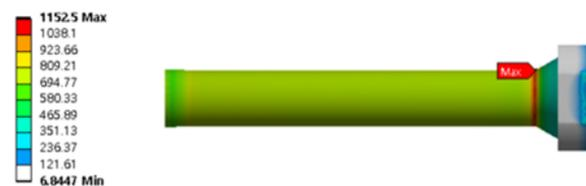
**Figure 6.** Von-mises stress of stem.
