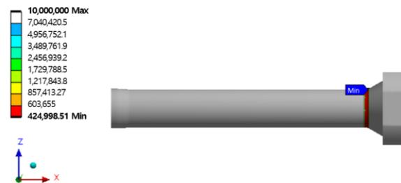
**Figure 24.** Results of the fatigue analysis of stem.
