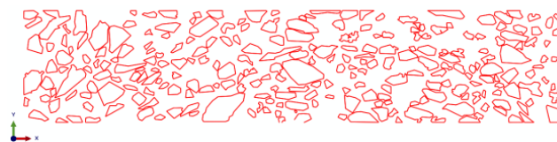
Figure 10. CZM elements between the aggregate and asphalt mortar.
