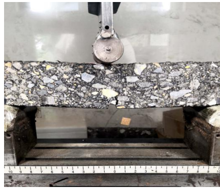
Figure 6. Bending failure of the beam specimen.
