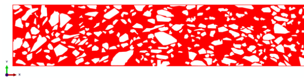
Figure 11. CZM elements inside of the asphalt mortar.
