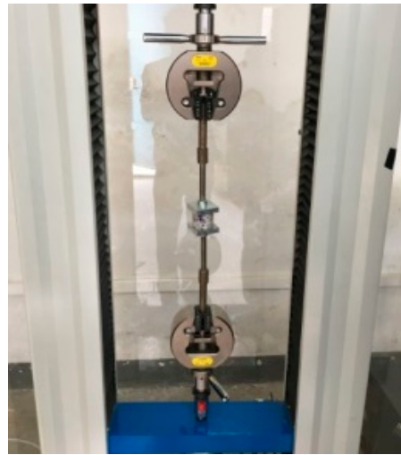
Figure 4. Bitumen bond strength (BBS) test.
