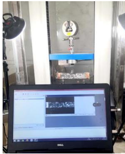
Figure 5. Three-point bending test.
