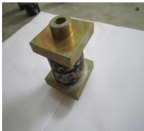
Figure 3. Sandwich specimen of the asphalt–aggregate bonding interface.
