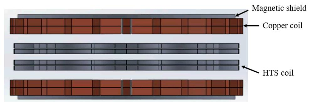
Figure 2. The structure of the axial flux HTS motor.
