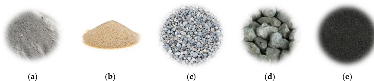
**Figure 1.** Test materials: (a) cement; (b) sand; (c) coarse aggregate; (d) recycled aggregate; (e) rubber granules.
