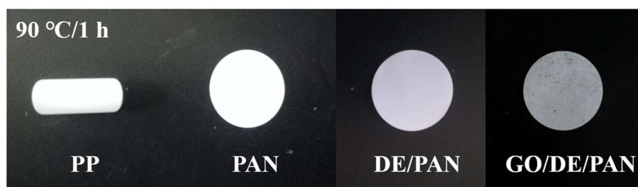
**Figure 6.** Images of the PP, PAN, DE/PAN, and GO/DE/PAN separators after heating at  $90^\circ\text{C}$  for 1 h.
