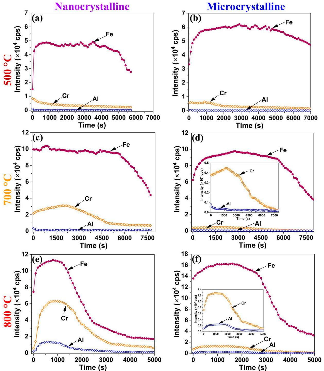
**Figure 7.** TOF-SIMS depth profiles of oxides formed on Fe-10Cr-3Al alloy in 60 h of oxidation of NC alloy at (a) 500 °C, (c) 700 °C, and (e) 800 °C and MC alloy at (b) 500 °C, (d) 700 °C, and (f) 800 °C.
