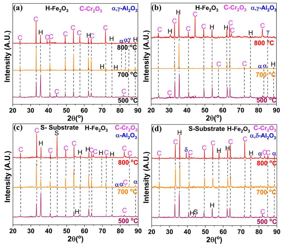
**Figure 5.** XRD profiles of oxide scales formed on (a) NC Fe-10Cr-5Al alloy, (b) MC Fe-10Cr-5Al alloy, (c) NC Fe-10Cr-3Al alloy and (d) MC Fe-10Cr-3Al alloy at 500, 700, and 800 °C in 60 h of oxidation.
