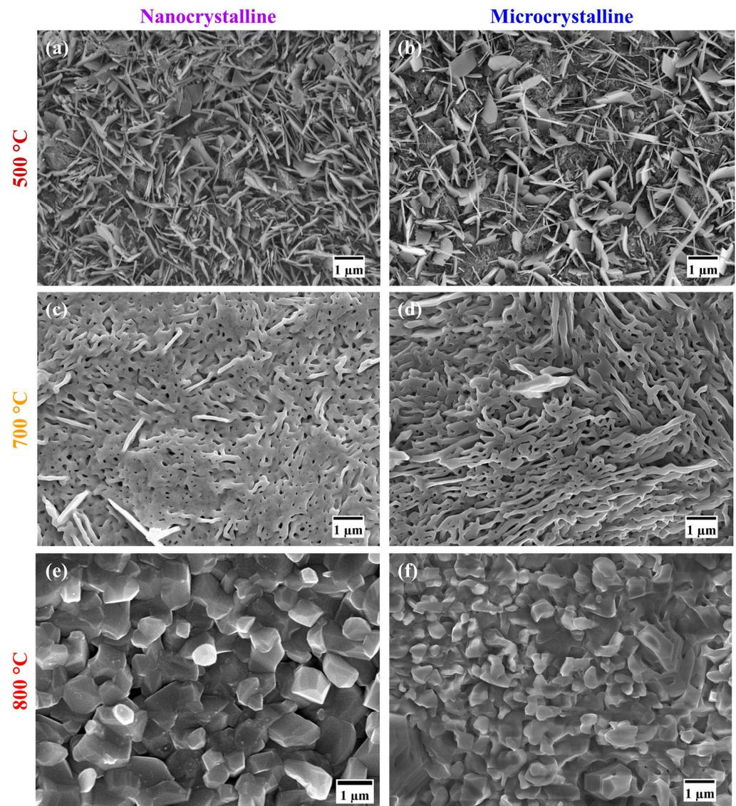
**Figure 4.** Morphologies of the oxide scales formed on the Fe-10Cr-3Al alloy in 60 h of the oxidation of the NC alloy at (a) 500 °C, (c) 700 °C, and (e) 800 °C and MC alloy at (b) 500 °C, (d) 700 °C, and (f) 800 °C.
