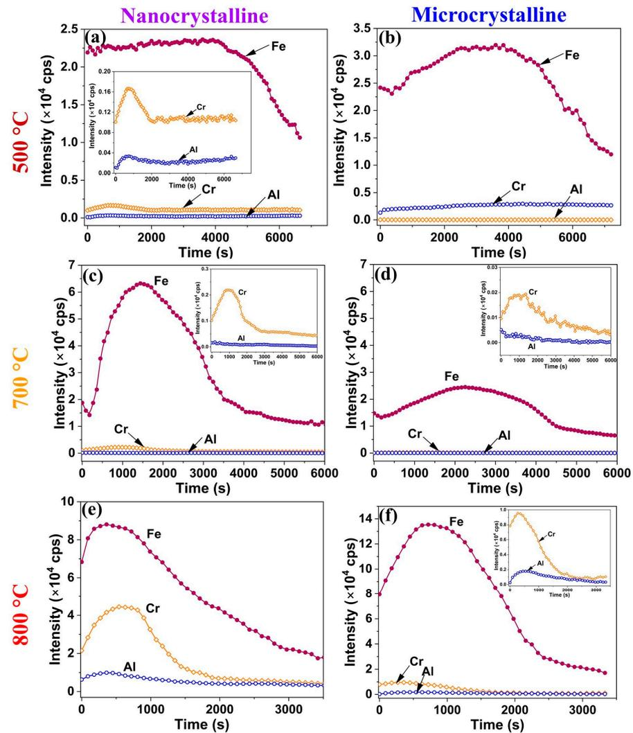
**Figure 6.** TOF-SIMS depth profiles of oxides formed on Fe-10Cr-5Al alloy in 60 h of oxidation of NC alloy at (a) 500 °C, (c) 700 °C, and (e) 800 °C and MC alloy at (b) 500 °C, (d) 700 °C, and (f) 800 °C.
