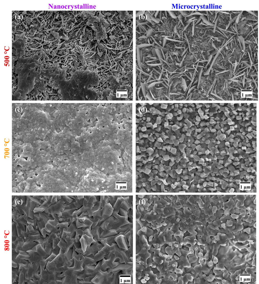
**Figure 3.** Morphologies of the oxide scales formed on the Fe-10Cr-5Al alloy in 60 h of the oxidation of the NC alloy at (a) 500 °C, (c) 700 °C, and (e) 800 °C and MC alloy at (b) 500 °C, (d) 700 °C, and (f) 800 °C.
