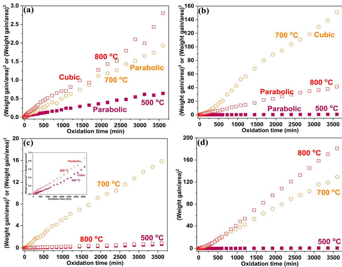
**Figure 2.** Oxidation kinetic plot for (a) NC Fe-10Cr-5Al, (b) MC Fe-10Cr-5Al, (c) NC Fe-10Cr-3Al, and (d) MC Fe-10Cr-3Al alloys oxidized at 500, 700, and 800 °C. The unit of weight gain/area is mg/cm<sup>2</sup>. If the (weight gain/cm<sup>2</sup>)<sup>2</sup> versus oxidation time curve is linear, then the alloys follow parabolic laws; the alloys follow cubic laws if the (weight gain/cm<sup>2</sup>)<sup>3</sup> versus oxidation time curve is linear.
