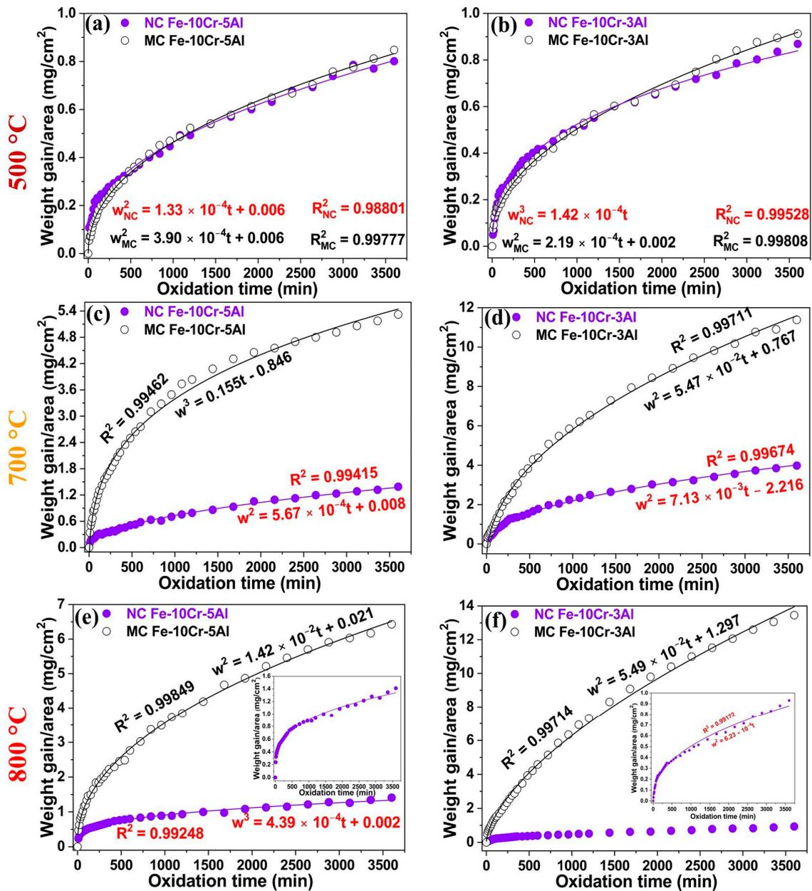
Figure 1. Oxidation kinetic plots for the Fe-10Cr-5Al alloy oxidized at (a) 500 °C, (c) 700 °C, and (e) 800 °C (inset, NC alloy) for 60 h. Oxidation kinetic plots for the Fe-10Cr-3Al alloy oxidized at (b) 500 °C, (d) 700 °C, and (f) 800 °C (inset, NC alloy) for 60 h.
