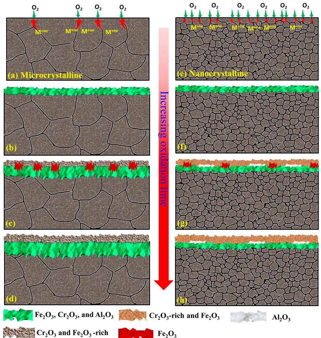
**Figure 8.** Schematic of plausible mechanism for oxide scale formation on microcrystalline (a–d) and nanocrystalline (e–h) Fe-10Cr-(3,5) Al alloys at high temperatures.
