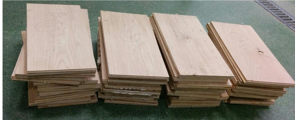
**Figure 2.** Samples prepared for static bending tests.
