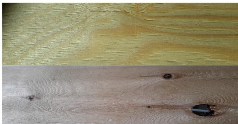
**Figure 1.** Examples of veneers in classes A (top) and D (bottom).
