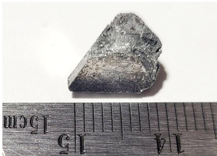
**Figure 1.** A single crystal of  $\text{YbCo}_{1.86}\text{Ni}_{0.14}\text{Zn}_{20}$  synthesized using the flux growth method.
