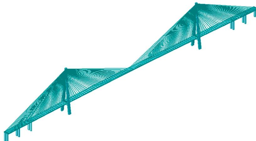
**Figure 8.** Finite element model of Sutong bridge.
