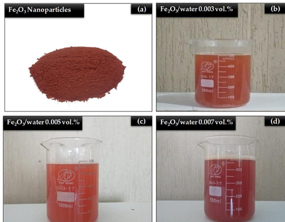
**Figure 12.** Samples of nanofluids (a) Ferric oxide nano powder, (b) nanofluid with 0.003 vol%, (c) nanofluid with 0.005 vol%, and (d) nanofluid with 0.007 vol% [164].
