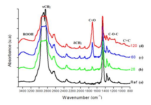
**Figure 4.** (a) FTIR spectra in the carbonyl (C=O) region of reference UHMWPE and UHMWPE submitted to peroxide accelerated ageing for different periods of time: (b) 7 days; (c) 14 days; (d) 21 days; (e) 28 days; (f) 60 days and (g) 120 days.
