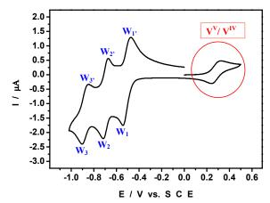
Figure 3A displays the CV obtained in pure pH = 5 medium. The potential domain was selected to avoid oxidation of Pd<sup>0</sup> nanostructures. The redox activity of the V<sup>V</sup>/V<sup>IV</sup> moiety is unambiguously
