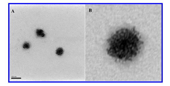
Figure 1. (A) Representative TEM of Pd<sup>0</sup>@POM blackberries and (B) an enlarged image.
