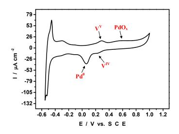
**Figure 6.** Cyclic voltammograms run at two different pH values with a Pd<sup>0</sup>@POM glassy carbon-modified electrode. The potential excursion was restricted to the domain where Pd<sup>0</sup> electro-oxidation does not occur. The scan rate was 10 mV s<sup>-1</sup>; reference electrode was SCE. (red) pH = 1; (blue) pH = 5.
