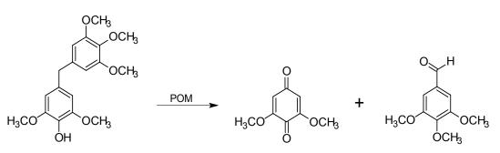
Figure 8. Degradation of a phenolic diphenylmethane with POMs [25].
