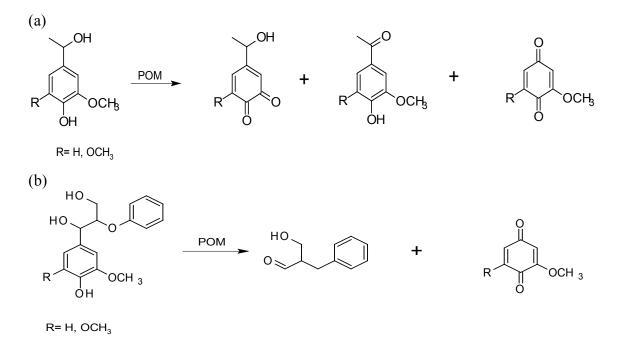
In addition to quinone formation confirmed in different model studies and studies on MWL and kraft pulps, an increase in other carbonyl groups, such as  $-C_{\alpha}HO$  and  $-C_{\alpha} = O$ , has been observed in the remaining POM-treated MWL and residual lignin of kraft pulps [28,34]. This result corroborates a reaction mechanism based on the successive oxidations of the benzylic carbon atoms, as proposed in the studies on etherified LMCs [26].
