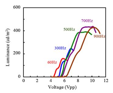
**Figure 8.** Frequency dependence of luminance characteristic to the voltage applied.
