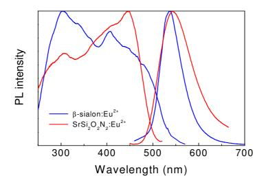
Figure 3. Excitation and emission spectra of green-emitting  $\beta$ -sialon:Eu<sup>2+</sup> and SrSi<sub>2</sub>O<sub>2</sub>N<sub>2</sub>:Eu<sup>2+</sup>.
