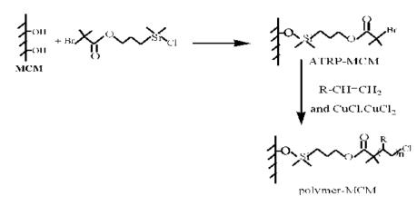
Figure 2. ATRP method for grafting polymer onto the mesoporous silica.
