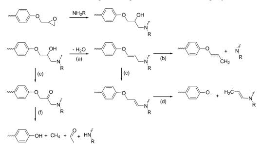
Scheme 2. Thermal degradation paths of an amine cured epoxy resin.
