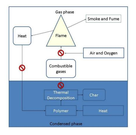
**Scheme 3.** Combustion cycle of a polymer fire. Red marks represent the main approaches to extinguish a fire scenario.
