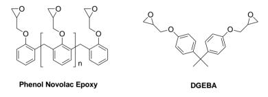
Epoxy resins in EE are commonly cured by reaction of the epoxy end group with amines (**a**), phenol novolac (**b**) or anhydrides (**c**) (Figure 3). The polyaddition of the hardener with the epoxy resin will then generate hydroxyl groups that can contribute to increasing the cross-linking density of the cured resin [10].
