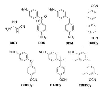
Figure 22. Hardeners used to cure epoxy resins (cf. Table 5).
