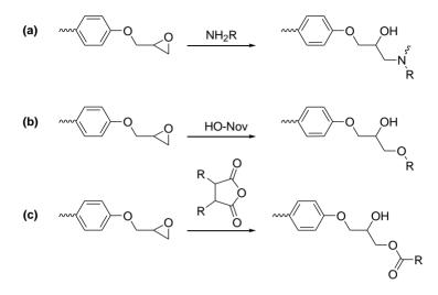
Different hardeners are used depending on the requirements of the application. In FR-4 laminates, dicyandiamide (DICY) and phenol novolac (PN) are mostly used (Figure 4) [5].
