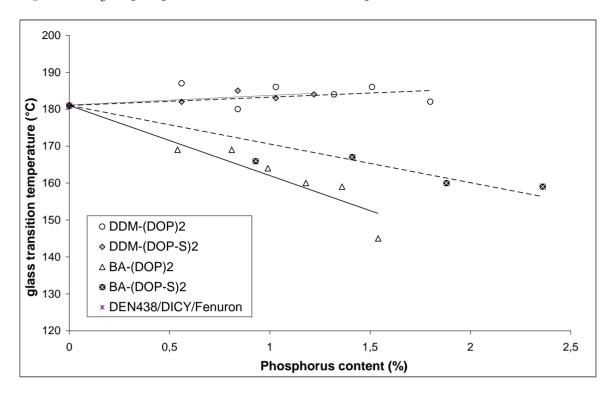
Figure 14. T<sub>g</sub> vs. phosphorus content of DEN438 samples cured with DICY/Fenuron [52].
