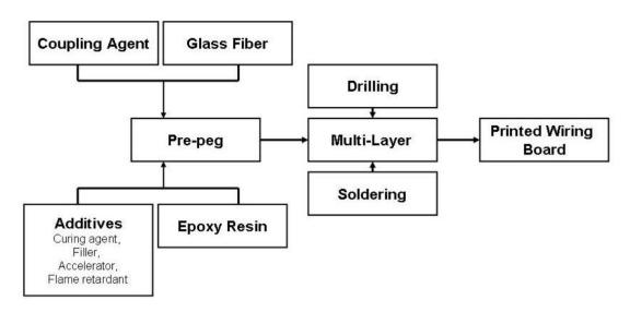
Scheme 1. Assembly fabrication of FR-4 printed wiring boards.
