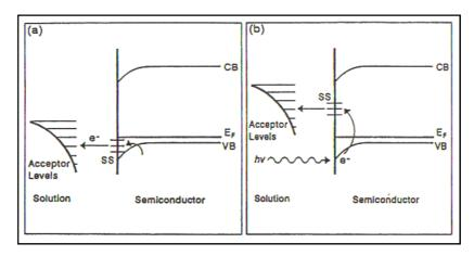
**Figure 8.** A schematic representation of a *p*-type semiconductor/solution interface (Reprint from [29] and [33]).
