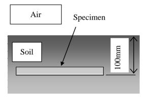
**Figure 3.** Schematic illustration of the biodegradable test (Condition 2).
