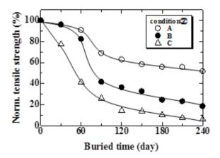
**Figure 8.** Relationship between normalized tensile strength and composting time under Condition 3 and 4.
