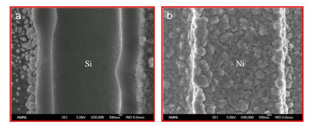
**Figure 4.** FESEM cross-sectional micrographs of the plated sidewalls at a depth of about 100  $\mu$ m, taken from different samples with various degrees of treatment: (a) 1-h metallization stage; (b) 2-h metallization stage; (c) 8-h metallization stage; (d) Enlarged image of the aggregated Ni deposits.
