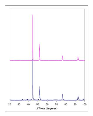
Figure 6. XRD spectra of pure Ni (upper) and an 8-hour wet treated sample (lower)
