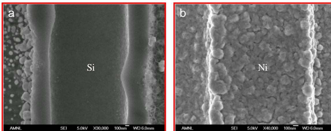
**Figure 4.** FESEM cross-sectional micrographs of the plated sidewalls at a depth of about 100  $\mu\text{m}$ , taken from different samples with various degrees of treatment: (a) 1-h metallization stage; (b) 2-h metallization stage; (c) 8-h metallization stage; (d) Enlarged image of the aggregated Ni deposits.
