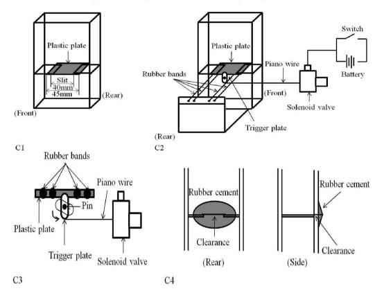
Figure A2. Apparatus for instant opening of slit.
