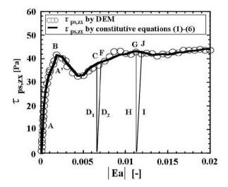
For confirmation, the stresses obtained by the constitutive equations with these functions are compared with the stresses obtained by DEM in Figure 2. It is not surprising that good agreement is obtained. Figures 1 and 2, and Appendix B describe the main features and asymptotic behavior of A1–A4 and the strain rate-independent stress  $\tau_{ps}$ .
