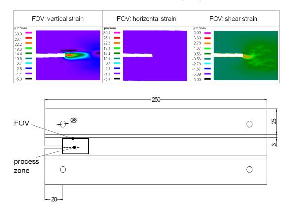
As described in Rathke *et al.* [4] and Sinn *et al.* [24], the deformation of the sample surface causes a change in the phase difference and therefore a new speckle pattern. To calculate an image with the
