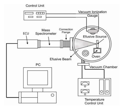
**Figure 1.** Molecular beam—thermal desorption mass spectrometer (MB-TDS) (Adapted from [6]).
