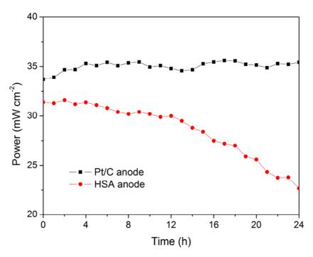
In addition, Figure 4 shows the HSA anode MEA electric performances and comparison with the Pt/C anode MEA.
