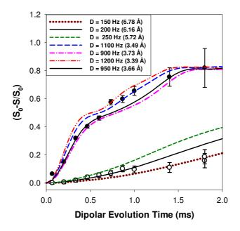
The <sup>1</sup>H-<sup>7</sup>Li REDOR MAS NMR buildup curves for the p15AA-45%Li and the r15AA-31%Li ionomer materials are shown in Figure 5. For these materials the individual proton environments were not as cleanly resolved during the REDOR experiments due to the reduced intensity of the more shielded component. Therefore, the REDOR buildup curves were obtained by integration of the entire
