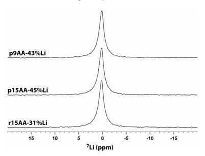
Figure 8. <sup>7</sup>Li MAS NMR of partially Li-neutralized P(E-AA) ionomers.
