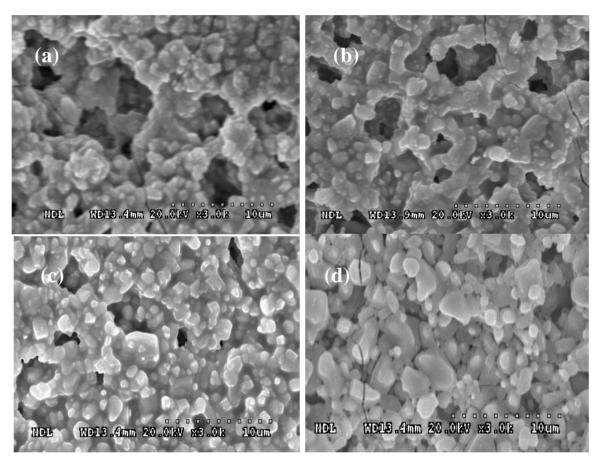
**Figure 5.** The SPTB layer/p-type Si(100) substrates were fired at 840  $^{\circ}$ C for 60 min and textured in 1.7% KOH solution for 25 min. Then, surface morphologies and cross-section images of the SPTB layer/p-type Si(100) substrates etched in mixed HCl/H<sub>2</sub>O<sub>2</sub> solution at (**a**,**b**) 10, (**c**,**d**) 30, (**e**,**f**) 60 min, respectively, were detected by SEM.
