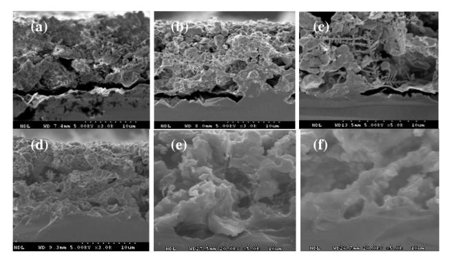
**Figure 3.** The SPTB layer/p-type Si(100) substrates were textured in 1.7% KOH solution for 25 min. (a) the surface morphology and (b) the cross-section image of the p-type Si(100) substrate without a SPTB layer was detected by SEM.
